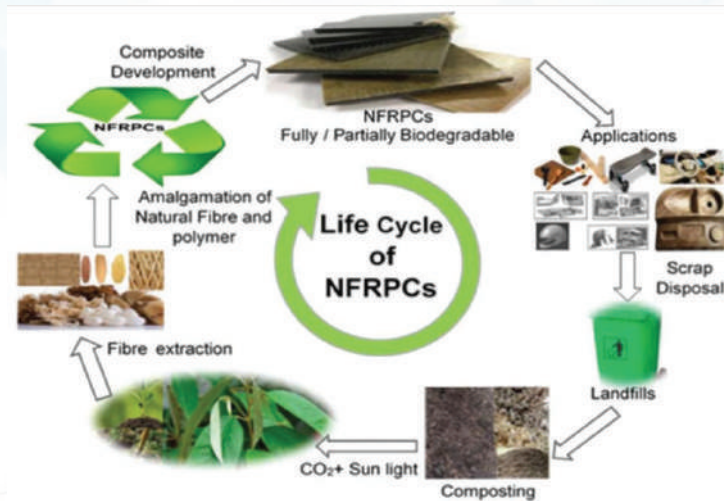
FIGURE 3. Life Cycle of Natural fiber reinforced composites [7]
